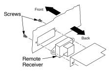
Figure 19 - Installing Remote Receiver
